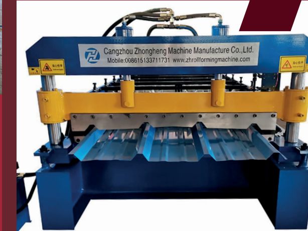
CORRUGATED SHEETS FORMING
